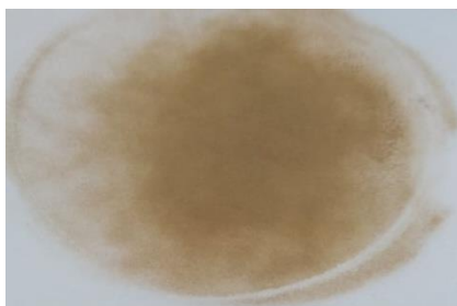
Figure 4. 8: A photograph of CDN after milling and sieving.
