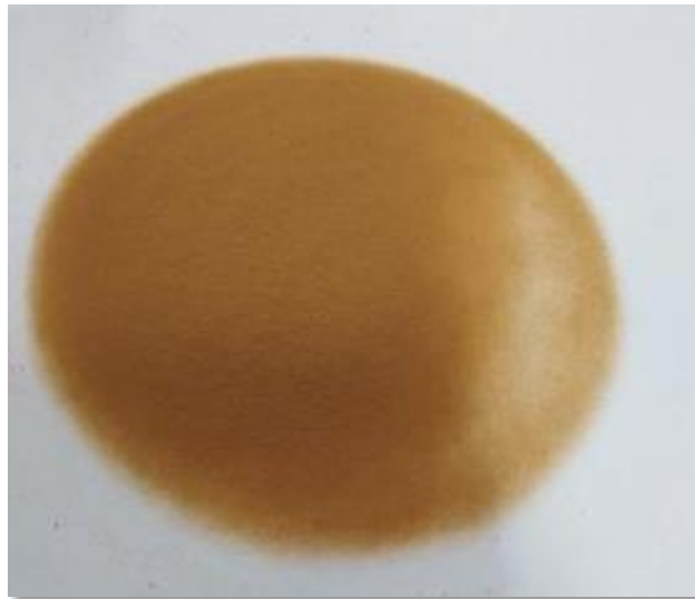
Figure 4. 5: A photograph of the date fruit powder showing a very cohesive powder after sieving (particle size less than 32 \mu m).
