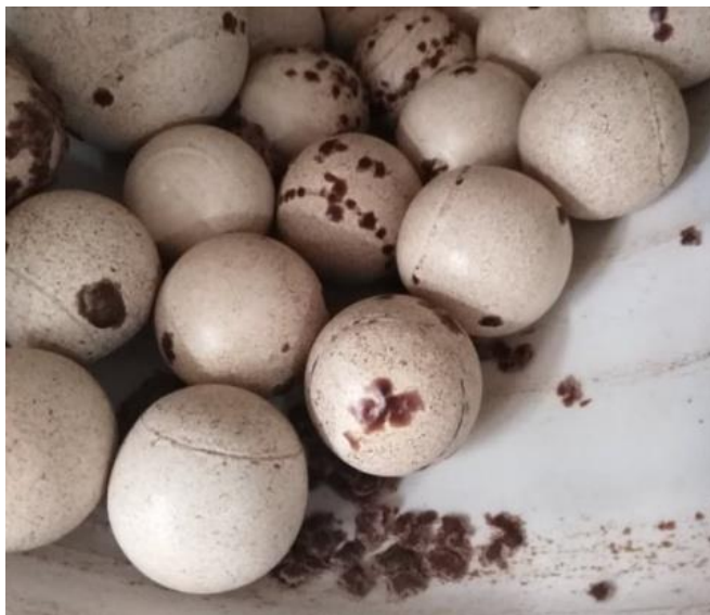
Figure 4. 6: A photograph of the date powder during ball milling highlighting the effect of excessive milling time formed solid cohesive pellets.
