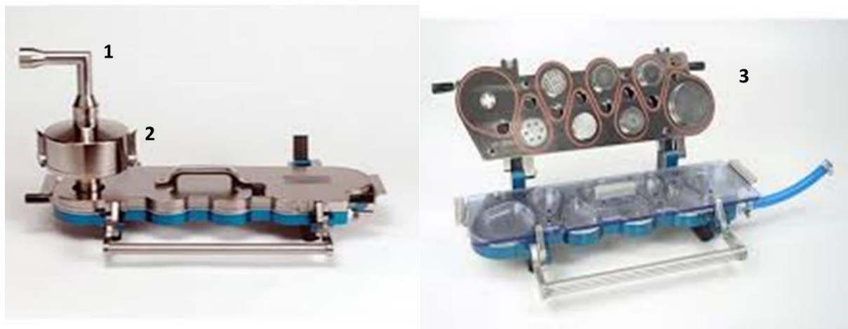
Figure 3. 2: A photograph of the next Generation Impactor highlighting its components. (1): induction tube, (2) pre-separator, (3) collection trays 1-8.
