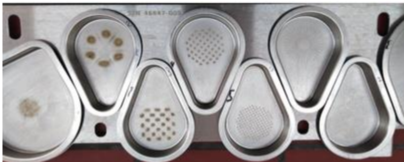
Figure 4. 11: Deposition of the chitosan date nanoparticles onto the NGI apparatus highlighting the brown powder from tray 1-7
