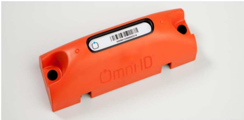
Figure 2-7: Active RFID Tag (Smiley, 2019)
