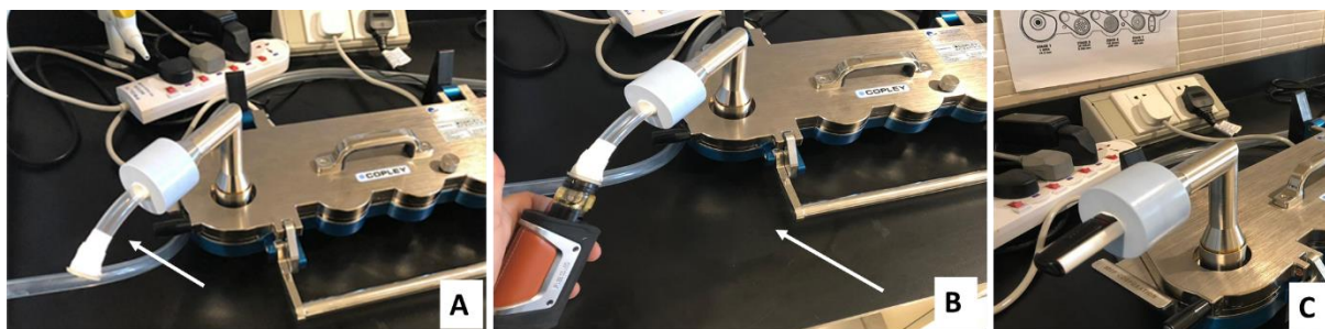
Figure 4. 6: Assembly for connection of the vapes to the NGI equipment to enable testing it. (A) the adaptor to the mouth piece to be used with vape tank (white arrow) and vape coil, (B) the adaptor connected to the vape tank (white arrows), (C) the pod does not require special custom made adaptor and fits well in the mouth piece.
